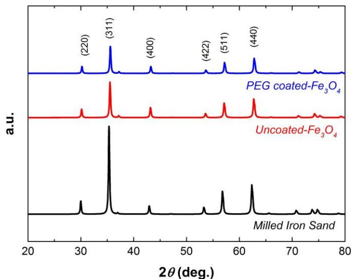
**Figure 1.** X-ray Diffraction pattern (XRD) of milled iron-sand, uncoated and PEG-coated  $\text{Fe}_3\text{O}_4$  samples.
