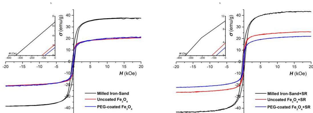
**Figure 4.** Hysteresis Curve of milled iron-sand, nano-Fe<sub>3</sub>O<sub>4</sub> and PEG-coated Fe<sub>3</sub>O<sub>4</sub> at powder condition (a) and as a magnetic elastomer (b).
