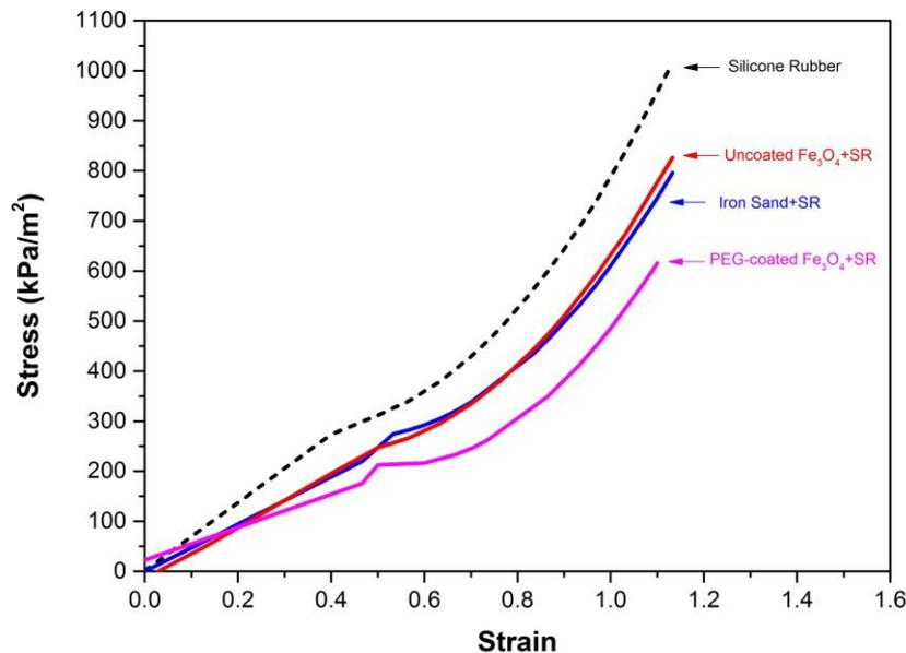
**Figure 3.** Stress-Strain analysis of elastomer material made of 100% silicone rubber (SR), 20% SR + uncoated  $\text{Fe}_3\text{O}_4$ , 20% SR + PEG-coated  $\text{Fe}_3\text{O}_4$ , and 20% SR + Milled iron-sand
