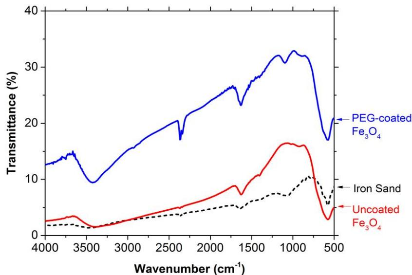
**Figure 2.** FTIR analysis of the samples: milled iron-sand, uncoated- $\text{Fe}_3\text{O}_4$ , and PEG-coated  $\text{Fe}_3\text{O}_4$ .
