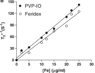
Figure 3. (A)  $1/T_2$  and (B)  $1/T_2^*$  versus Fe concentration for PVP-IO ( $\bullet$ ) and Feridex ( $\circ$ ). The relaxivity values  $r_2$  and  $r_2^*$  were obtained from the slopes of the linear fits of experimental data.
