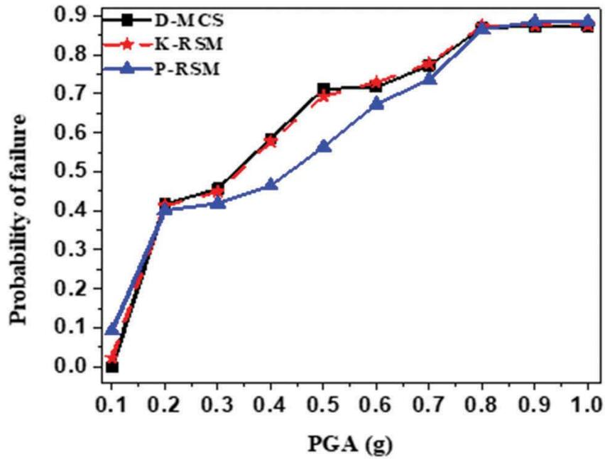
Figure 12. Comparison of fragility of the RC frame at LS level.
