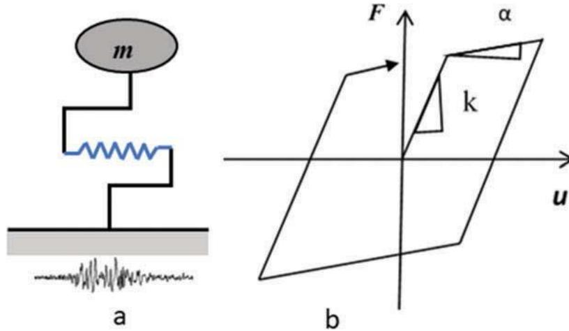
**Figure 1.** (a) The spring mass system and (b) the force deformation behavior of the nonlinear spring.
