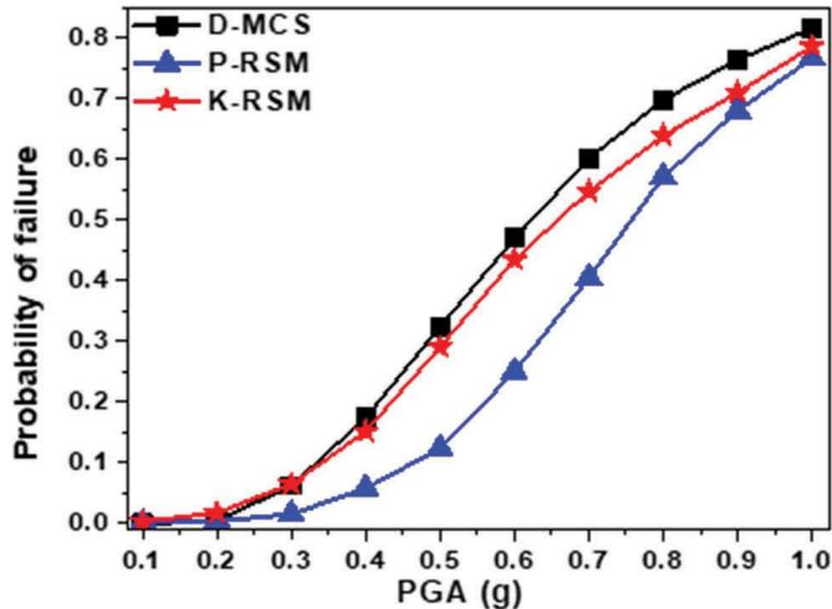
**Figure 4.** Comparison of fragility of the SDOF system by the proposed K-RSM and the P-RSM based on the direct response approximation approach.
