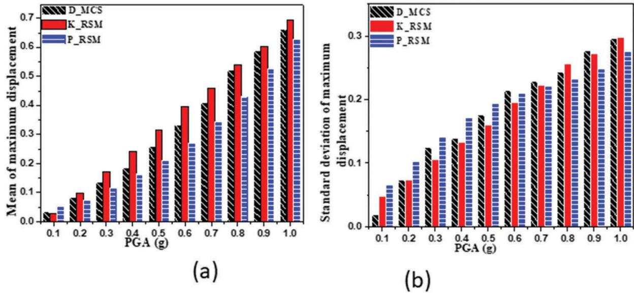
**Figure 3.** (a) Comparison of (a) the mean and (b) the standard deviation of the maximum displacement by the K-RSM and the P-RSM based on the proposed direct response approximations approach.
