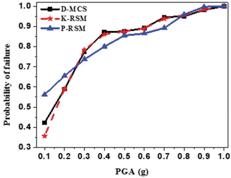
Figure 11. Comparison of fragility of the RC frame at IO level.
