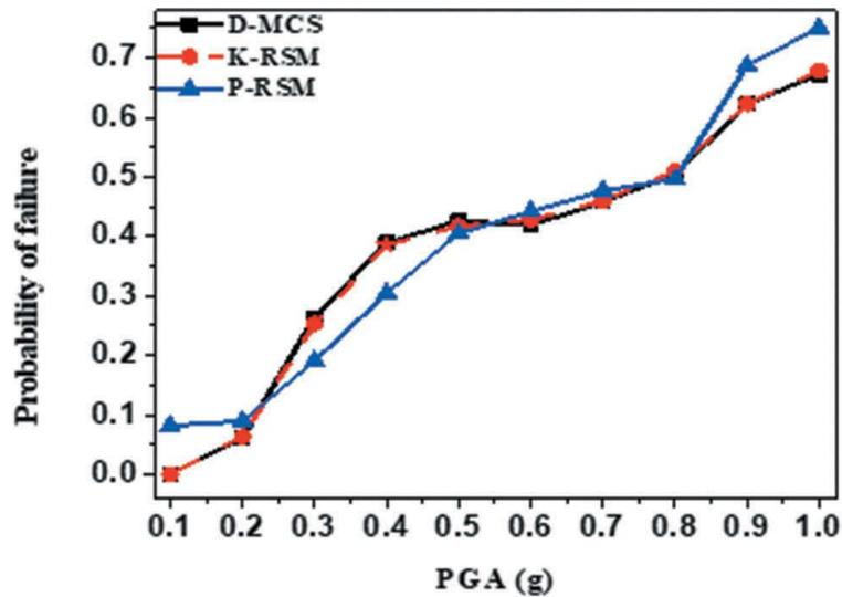
**Figure 13.** Comparison of fragility of the RC frame at CP level.
