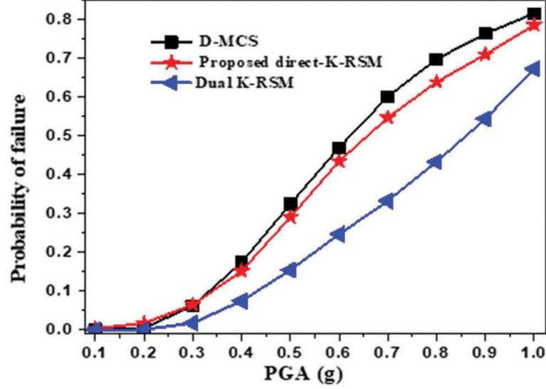
**Figure 2.** Comparison of fragility of the SDOF system by the dual K-RSM and the proposed direct K-RSM approaches.
