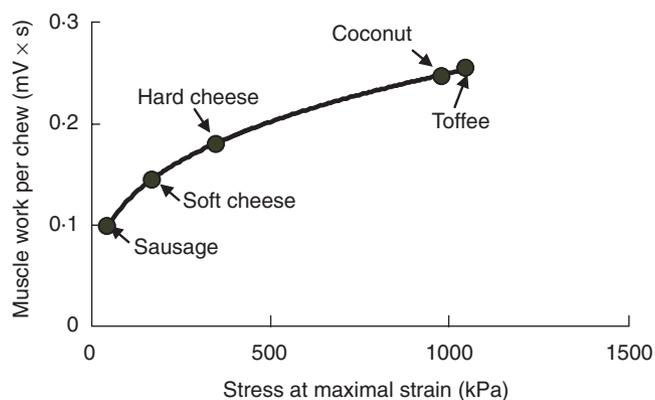
**Fig. 1.** Relationship between mean muscle work per chew recorded by electromyography during chewing and the stress at maximal strain measured by compression test in an Instron machine from five different products ( $y = 0.0298x^{0.3077}$ ;  $R^2$  0.999). Values are means from thirty-six subjects. (From Mioche *et al.* 1999.)
