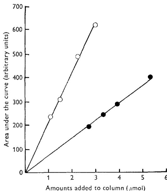
Fig. 1. Relationships between eluted peak areas and concentrations of materials chromatographed on Sephadex G-10. Samples (2 ml) of solutions containing adenosine (○) or guanine (●) were applied to a 900 mm  $\times$  15 mm Sephadex G-10 column and eluted under conditions described on p. 333.
