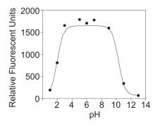
**Fig. 6.** The fluorescence emission of HO-Mito-Etd<sup>+</sup> in the presence of 0.17  $\mu$ g of DNA as a function of pH ( $\lambda_{ex} = 396$  nm;  $\lambda_{em} = 579$  nm). This curve was fit to find two pK<sub>a</sub>s at 2.1 and 10.5, and a third pK<sub>a</sub> was determined to be 0.65 by plotting the fluorescence emission at 795 nm with  $\lambda_{ex} = 396$  nm (not shown). Fluorescence of HO-Mito-Etd<sup>+</sup> is maximal and independent of pH over the physiological range.
