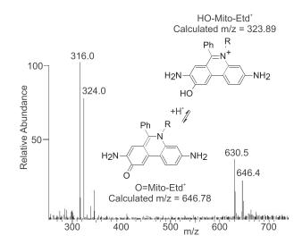
**Fig. 5.** Mito-HE oxidized by xanthine/xanthine oxidase was analyzed by electrospray ionization and ion trap mass spectrometry. The ions at m/z = 316.0 and 630.5 were identified as Mito-Etd<sup>+</sup>. The doubly charged ion at m/z = 324.0 corresponded to the molecular weight of the hypothesized structure of HO-Mito-Etd<sup>+</sup>. The singly charged ion at m/z = 646.0 lead to the proposal of the carbonyl structure, O=Mito-Etd<sup>+</sup>.
