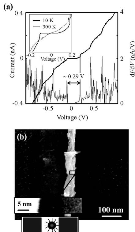
FIG. 3. (a) Current-voltage curves obtained at the nanogap device after the dispersion of Au nanoparticles. The Coulomb staircase is clearly observed. Enlarged graph near  $V=0 \text{ V}$  is also shown in the inset. (b) SEM image of the nanogap electrodes from which the  $I$ - $V$  curve shown in (a) was taken. The single nanoparticle was placed to make an asymmetric junction between the two electrodes.
