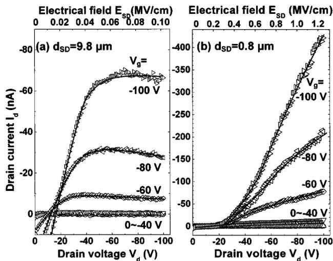
FIG. 2. Drain current ( $I_d$ ) vs drain voltage ( $V_d$ ) characteristics depending on channel length between source and drain electrodes,  $d_{SD}=9.8 \mu\text{m}$  (a) and  $0.8 \mu\text{m}$  (b), in OLEFETs with TPTPT layer as active layer. Various gate voltages ( $V_g$ ), 0 V ( $\circ$ ), -20 V ( $\Delta$ ), -40 V ( $\nabla$ ), -60 V ( $\diamond$ ), -80 V ( $\triangleleft$ ) and -100 V ( $\triangleright$ ), were applied in these devices.
