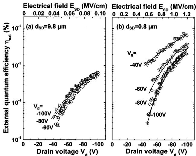
FIG. 4. External quantum efficiency ( $\eta_{\text{ext}}$ ) vs drain voltage ( $V_d$ ) characteristics depending on channel length between source and drain electrodes,  $d_{\text{SD}}=9.8 \mu\text{m}$  (a) and  $0.8 \mu\text{m}$  (b), in OLEFETs with TPTPT layer as active layer. Various gate voltages ( $V_g$ ),  $-40 \text{ V}$  ( $\nabla$ ),  $-60 \text{ V}$  ( $\diamond$ ),  $-80 \text{ V}$  ( $\triangleleft$ ) and  $-100 \text{ V}$  ( $\triangleright$ ), were applied in these devices.
