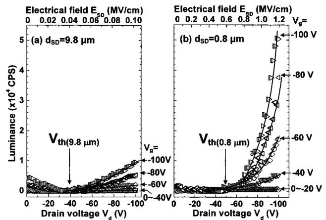
FIG. 3. Luminance ( $L$ ) vs drain voltage ( $V_d$ ) characteristics depending on channel length between source and drain electrodes,  $d_{SD}=9.8 \mu\text{m}$  (a) and  $0.8 \mu\text{m}$  (b), in OLEFETs with TPTPT layer as active layer. Various gate voltages ( $V_g$ ), 0 V ( $\circ$ ), -20 V ( $\Delta$ ), -40 V ( $\nabla$ ), -60 V ( $\diamond$ ), -80 V ( $\triangleleft$ ) and -100 V ( $\triangleright$ ), were applied in these devices.
