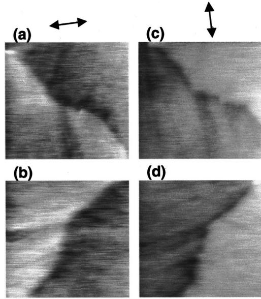
FIG. 3. Directional shear force images ( $2.4 \times 2.4 \mu\text{m}^2$ ) of one region of a PDA monolayer. (a) With  $+y, -x$  drive (direction shown at top with respect to image) and  $0^\circ$  scan angle. (b) Same as (a), except  $90^\circ$  scan angle. (c) With  $+y, +x$  drive (direction shown at top with respect to image) and  $0^\circ$  scan angle. (d) Same as (c), except  $90^\circ$  scan angle.
