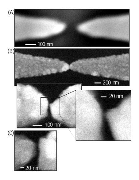
Figure 2 Scanning electron microscope (SEM) images before and after electrodeposition (scale bars show dimensions). (A) Electrodes before electrodeposition. (B) Electrodes after electrodeposition. The resolution of the SEM is 5 nm, not sufficient to resolve the gap. (C) Electrodes in which the gap was re-opened by electrodissolution, by reversing  $V_{dc}$  following an intentional short-circuiting (contacting) in a previous electrodeposition process.
