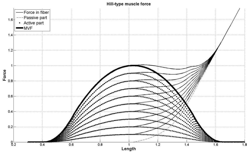
**Figure 1. Force-length relations in Hill-type muscle models: Changes in activation levels are associated with a group of contractile force curves (dotted curves); the addition of passive properties (dashed curve) provides the global force-length curves (solid curves)**
