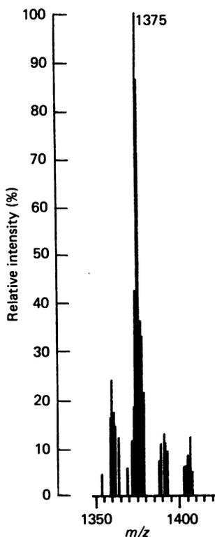
Fig. 8. Positive-ion mass spectrum of fraction 7
