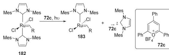
Scheme 87 Visible-light-controlled ruthenium-catalyzed olefin metathesis.
