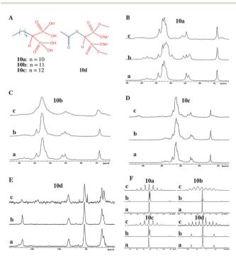
**Fig. 14** Bisphosphonate hydrogelators: (A) chemical structures of hydrogelators; (B–E) <sup>13</sup>C CP MAS NMR spectra of (a) synthetic solid; (b) xerogel and (c) gel (4 or 5 w/v%) of **10a–10d**; (F) <sup>31</sup>P CP MAS NMR spectra of (a) synthetic solid; (b) xerogel and (c) the hydrogel of **10a–10d**. Reproduced with permission from ref. 51, Copyright © 2013 Royal Society of Chemistry.
