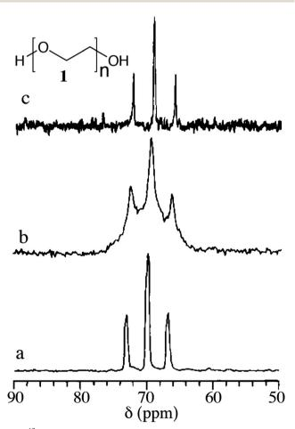
**Fig. 3** <sup>13</sup>C MAS solid state NMR spectra of polyethylene oxide (PEO, 1). (a) <sup>13</sup>C MAS NMR spectrum of gel containing 70% PEO and 30% of water at 4 kHz; (b) <sup>13</sup>C MAS NMR spectrum of gel containing 70% PEO and 30% of water in a static rotor and (c) <sup>13</sup>C NMR spectrum of 5% PEO solution in the liquid state probe. Reproduced with permission from ref. 36, Copyright © 1989 Elsevier Inc.
