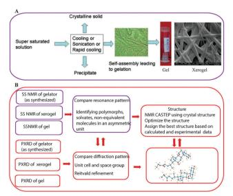
**Fig. 2** (A) The gelation mechanism of low molecular weight gelators. Reproduced with permission from ref. 43, copyright © 2010 Royal Society of Chemistry; (B) various steps involved in NMR crystallography of gels and gelators.
