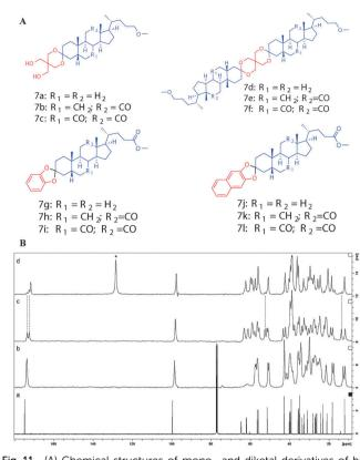
**Fig. 11** (A) Chemical structures of mono- and diketal derivatives of bile acids. (B) <sup>13</sup>C NMR spectrum of **7a** in CDCl<sub>3</sub> (a) and <sup>13</sup>C CP MAS NMR spectra of **7a** crystallized from acetonitrile (b), toluene (c), and benzene (d). Reproduced with permission from ref. 46, Copyright © 2010 Royal Society of Chemistry.
