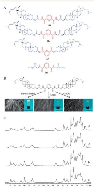
**Fig. 13** (A) Chemical structures of metallosupramolecular gelators. (B) Structure of compound **9a**, a gelator of the  $A(LS)_2$  type, with marked non-covalent interaction sites. (C)  $^{13}$ C CP MAS NMR spectra of (a) solid of **9a** from CHCl<sub>3</sub>; (b) xerogel of **9a** from pentan-1-ol; (c) xerogel of **9a** + Ag(i) from pentan-1-ol and (d) xerogel of **9a** + Zn(II) from pentan-1-ol. Reproduced with permission from ref. 48, Copyright © 2012 Royal Society of Chemistry.
