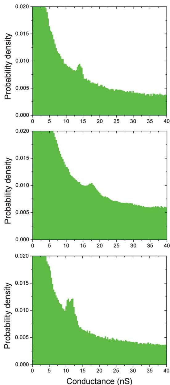
**Fig. 5** Single-molecule conductance modulation of cyt  $b_{562}$  SH-SA by its redox state. The redox state of the protein was controlled by the working substrate potentials applied: (top) the oxidised form ( $\eta = +300$  mV), (middle) the equilibrium state ( $\eta = 0$  mV), and (bottom) the reduced form ( $\eta = -300$  mV). The measurements were performed in 10 mM phosphate buffer (pH 6.2) at a fixed bias voltage of  $-0.1$  V.
