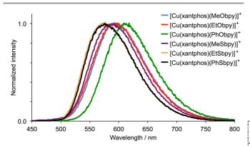
**Fig. 7** Emission spectra of [Cu(xantphos)(N^N)][PF<sub>6</sub>] complexes in frozen Me-THF ( $\lambda_{ext}$  = 410 nm).
