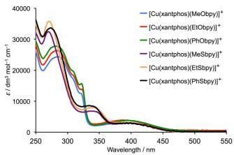
Fig. 4 Absorption spectra of  $CH_2Cl_2$  solutions of  $[Cu(xantphos)(N^N)][PF_6]$  complexes (concentration =  $2.5 \times 10^{-5}$  mol dm<sup>-3</sup>).
