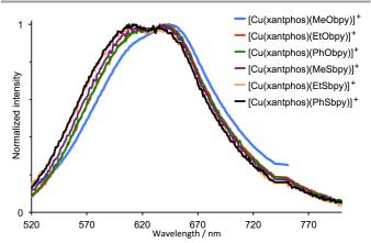
**Fig. 5** Emission spectra of solutions (CH<sub>2</sub>Cl<sub>2</sub>, 2.5  $\times$  10<sup>-5</sup> mol dm<sup>-3</sup>) of [Cu(xantphos)(N^N)][PF<sub>6</sub>] complexes (see Table 6 for  $\lambda_{exc}$ ).
