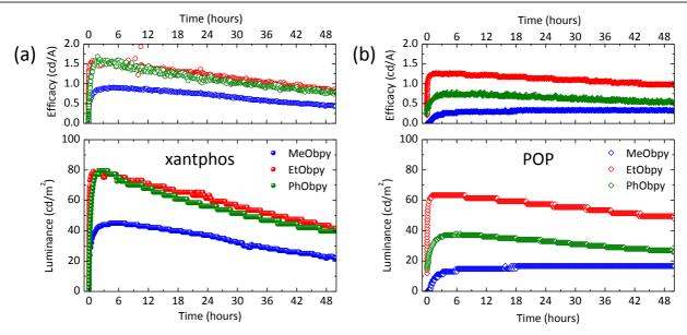
Fig. 8 Efficacy (top) and luminance (bottom) versus time for LECs employing Cu(I) complexes with RObpy and either (a) xantphos or (b) POP ligands. LECs were driven at an average current density of 50 A m<sup>-2</sup>.
