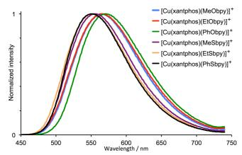
**Fig. 6** Emission spectra of powder samples of [Cu(xantphos)(N^N)][PF<sub>6</sub>] complexes ( $\lambda_{exc}$  = 365 nm).
