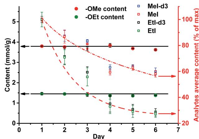
Fig. 9 Content of OMe and OEt groups determined in organosolv lignin (left axis) and the stability of the individual analytes (Mel/Mel-d<sub>3</sub> and EtI/EtI-d<sub>5</sub>) remaining in test vials upon standing for six days at RT without neutralization (right axis).
