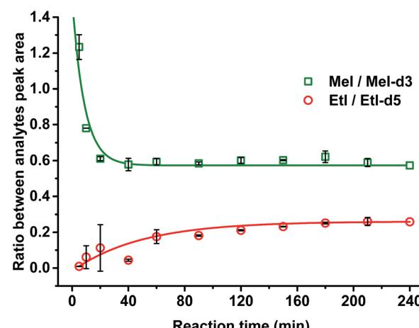
Fig. 4 Ratio between analytes (Mel/Mel-d<sub>3</sub> and Etl/Etl-d<sub>5</sub>) generated upon HI acid treatment from organosolv lignin and internal standards (4-(methoxy-d<sub>3</sub>)-benzoic acid and 4-(ethoxy-d<sub>5</sub>)-benzoic acid). Stabilization of the ratio between generated Etl and Etl-d<sub>5</sub> occurred after about 180 min.
