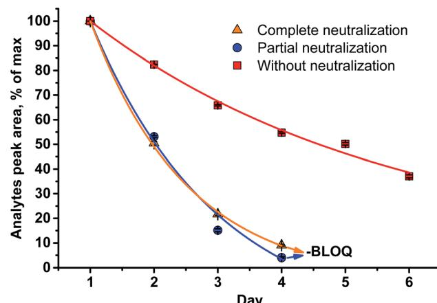
Fig. 6 Stability of the analytes (MeI/MeI-d<sub>3</sub>) generated in the reaction medium upon standing for six d at RT (LOQ = limit of quantification).
