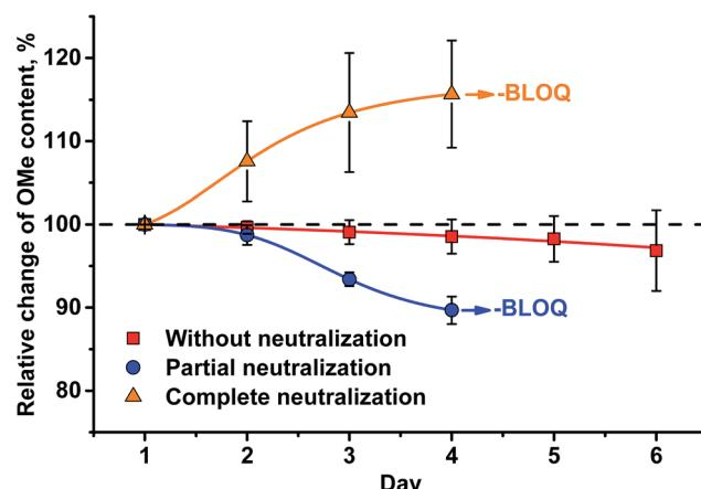
Fig. 7 Change of HS-ID GC-MS methoxyl group quantification when analytes (MeI/MeI-d<sub>3</sub>) remain in the test vials upon standing for six d at RT.
