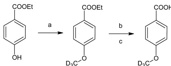
**Fig. 1** Synthesis of the internal standard 4-(methoxy-d<sub>3</sub>)-benzoic acid (2). Conditions: (a) CD<sub>3</sub>I, K<sub>2</sub>CO<sub>3</sub>, acetone, RT, 48 h; (b) NaOH, MeOH, H<sub>2</sub>O, reflux, 3 h; (c) HCl, H<sub>2</sub>O
