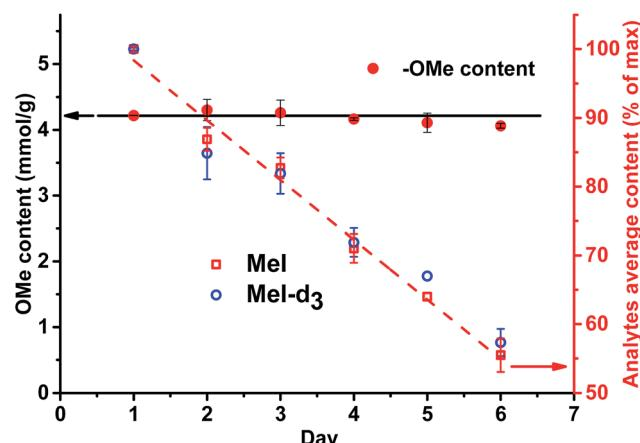
Fig. 8 Content of OMe group determination in kraft lignin (left axis) and stability of the analytes (Mel/Mel-d<sub>3</sub>) remaining in the test vials upon standing for 6 d at RT without neutralization (right axis).
