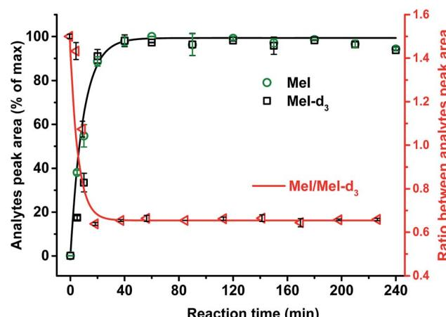
Fig. 3 Effect of HI acid treatment time on kraft lignin and internal standard (4-(methoxy-d<sub>3</sub>)-benzoic acid) on methoxyl groups conversion and formation of Mel and Mel-d<sub>3</sub>. Stabilization of the ratio between generated Mel and Mel-d<sub>3</sub> occurred after about 30 min.
