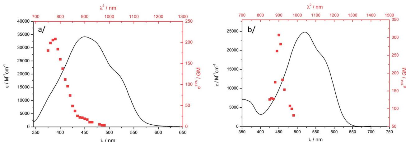
Fig. 7 Two-photon excitation spectra (■, higher x-coordinate and —, right y-coordinate) and OPA absorption spectra (—, lower x-coordinate and —, left y-coordinate) of particles in water: (a) **1** and (b) **2**.
