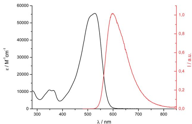
Fig. 4 Electronic absorption (conc.  $\approx 10^{-5}$  M, black) and corrected fluorescence emission (conc.  $\approx 10^{-6}$  M,  $\lambda_{\text{exc}}$  at the absorption maximum, red) spectra of **2** in DCM.
