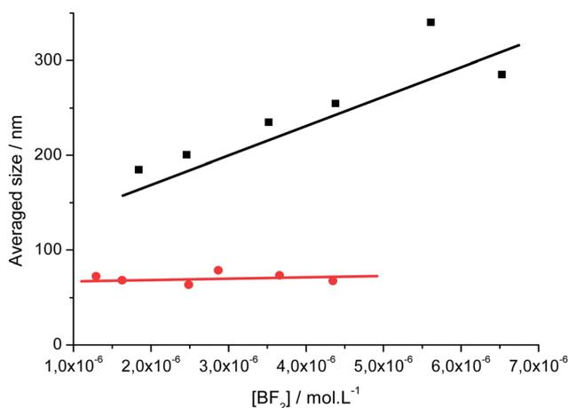
Fig. 2 Variation of the averaged size determined by DLS for dye 1 (black) and dye 2 (red) as a function of the total dye concentration.
