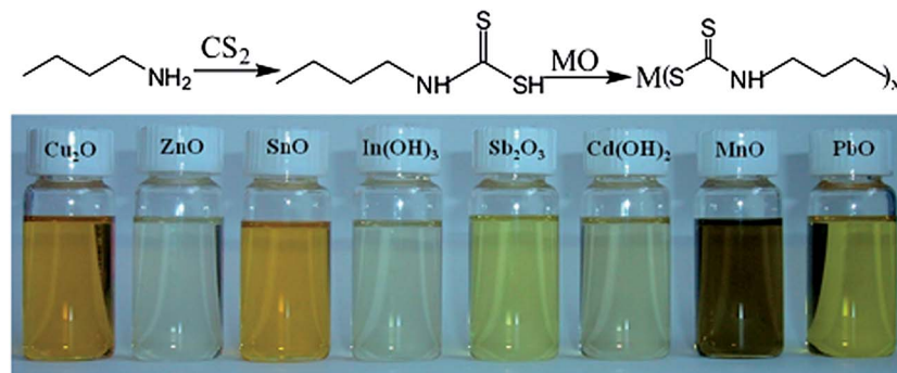
Fig. 9 (Top) Reaction mechanism of a metal oxide with butyldithiocarbamic acid. (Bottom) Digital photograph of various metal oxides dissolved in chloroform with the aid of butylamine and carbon disulfide ( \sim 0.35 M metal concentration). Reprinted with permission from ref. 73, Copyright 2012 American Chemical Society.
