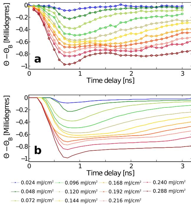
**Figure 3.** (a) The angular shifts  $\Theta - \Theta_B$  are calculated by taking the differences in the (0 0 4) diffraction peak centroid before and after the laser strikes the sample as a function of x-ray to laser delays for varying laser fluences. (b) Simulated angular shifts  $\Theta - \Theta_B$  for the (0 0 4) diffraction peak after effects of carrier saturation and TPA are incorporated, showing consistent results with the experimental data above.
