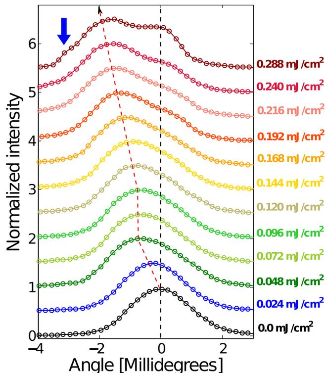
**Figure 4.** Bragg diffraction curves at various laser fluences (vertically offset) at  $\Delta t = 700$  ps for the n-doped GaAs sample. Black dashed line indicates the Bragg diffraction condition for an unperturbed crystal. Red dashed line shows centroid of the rocking curve up to laser fluence of  $0.048$  mJ/cm<sup>2</sup>, and then subsequently the centroids of the de-convolved peaks that come from the laser excited part of the crystal.
