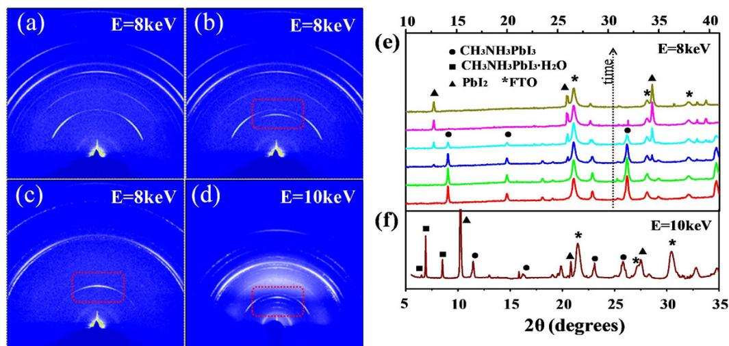
**Figure 2.** *In situ* XRD patterns. (a–d) Typical diffraction patterns of spin-coated  $\text{CH}_3\text{NH}_3\text{PbI}_3/\text{FTO}$  in degradation process and (e–f) the corresponding integral curves obtained by using Fit2D program.
