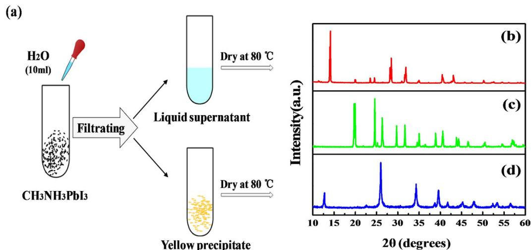
**Figure 4.** (a) Schematic diagram of solid-liquid separation experiment; XRD patterns of (b)  $\text{CH}_3\text{NH}_3\text{PbI}_3$  powder, (c) the resulting powder separated out from the liquid supernatant and (d) dried yellow precipitate.
