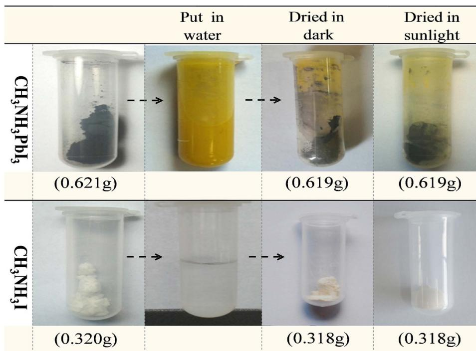
**Figure 5.** Color and weight change of  $\text{CH}_3\text{NH}_3\text{PbI}_3$  (1<sup>st</sup> row) and  $\text{CH}_3\text{NH}_3\text{I}$  (2<sup>nd</sup> row) powder when dried in dark or sunlight.
