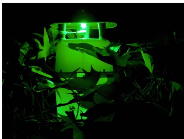
**Figure 2** | Solar powered green light funnel trap used in trials. A rubber septum, loaded with sweetpotato weevil male lure ((*Z*)-3-dodecenyl (*E*)-2-butenate) is attached to a side column of the trap to facilitate positioning the rubber septum immediately below the green light (photograph by Grant McQuate).
