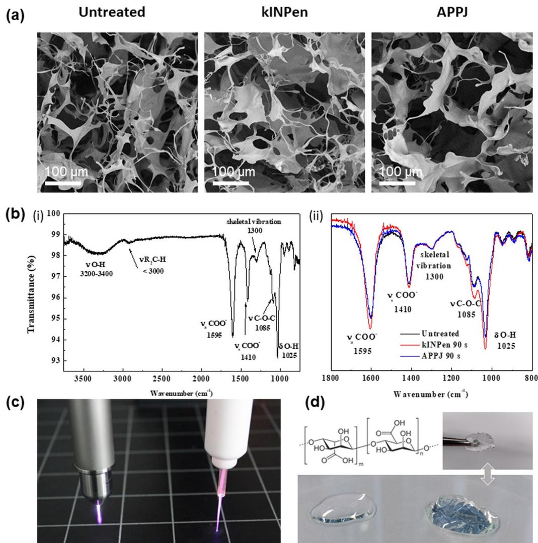
**Figure 3.** SEM micrographs (a) and FTIR-ATR spectra (b) of untreated (i), kINPen- and APPJ-treated 0.5% alginate for 90 s, at 10 mm distance and 1 L/min. Digital picture of kINPen and APPJ in operation (c). Chemical structure of alginate and digital pictures of the alginate solution (left side) and of the cross-linked alginate hydrogel (right side) (d).
