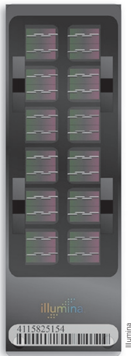
A sketch of the Human610-Quad chip, which contains 610,000 SNPs and 610,000 different bead types per array.
