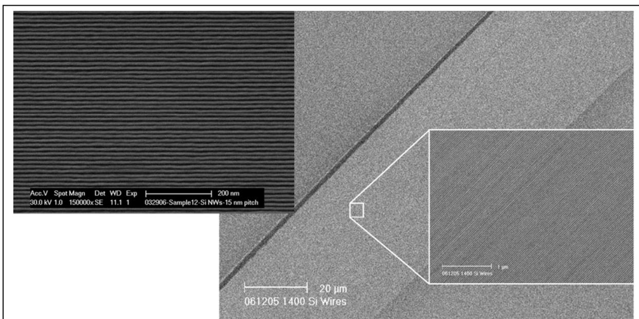
**Supplementary Figure 5 | The limits of SNAP patterning to produce high-density silicon NW arrays for crossbar circuit applications. (left)** An array of 7 nm wide Si NWs patterned at 6.5 nm half-pitch. **(right)** An array of 1400 Si NWs patterned at 16.5 nm half-pitch, providing enough NWs to produce an approximately 2 million bit crossbar circuit. The inset shows an expanded view of the array, which is virtually free of defective nanowires.
