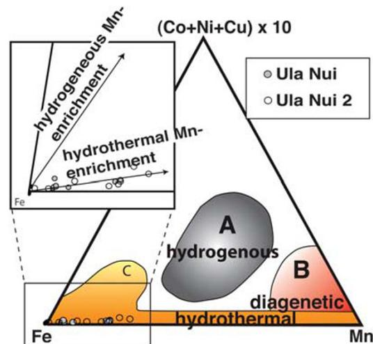
**Figure 3** Ternary diagram for Mn-Fe-(Co + Ni + Cu)  $\times 10$  in Ula Nui mats. The diagenetic, hydrothermal and hydrogenous fields are after Hein *et al.* (1994) and references therein. Ula Nui mat materials are inferred to be solely of hydrothermal origin.
