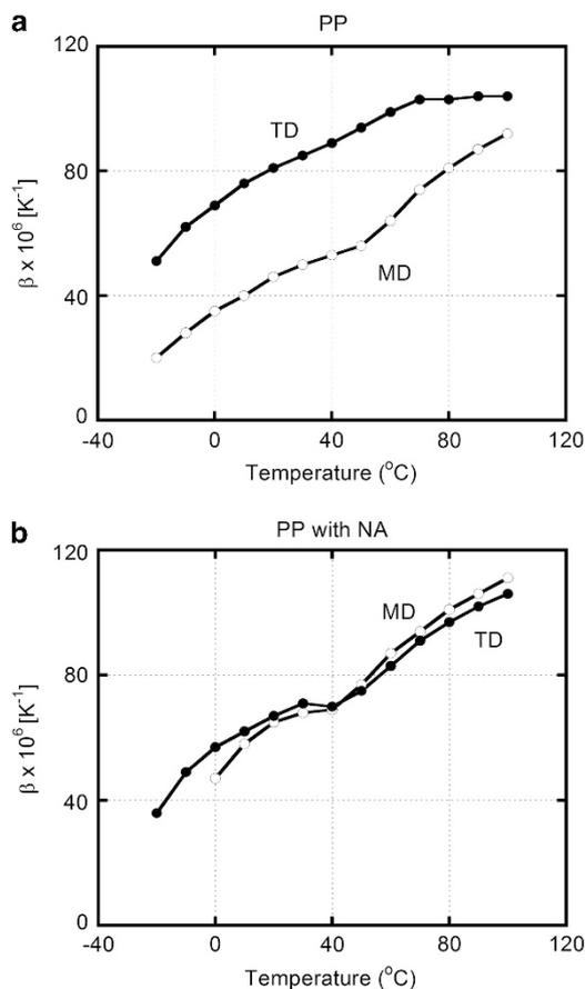
**Figure 8** Temperature dependence of linear coefficient of thermal expansion  $\beta$  in machine direction (MD; open symbol) and transversal direction (TD; closed symbol) directions for the injection-molded plates of (a) pure polypropylene (PP) and (b) PP containing the nucleating agent.
