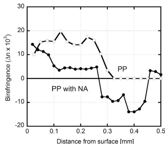
**Figure 2** Distribution of orientation birefringence for thin slices (parallel to machine direction (MD)– neutral direction (ND) plane) of pure polypropylene (PP; open symbol) and PP containing the nucleating agent (closed symbol). The identical data for PP containing the nucleating agent were reported previously.<sup>27</sup>
