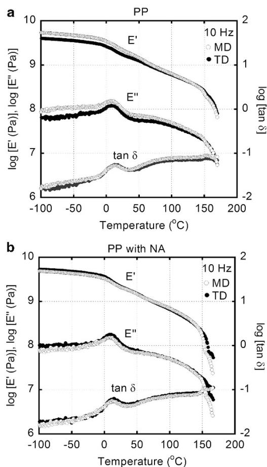
**Figure 6** Temperature dependence of tensile storage modulus  $E'$ , tensile loss modulus  $E''$ , and loss tangent  $\tan \delta$  in machine direction (MD; open symbols) and transversal direction (TD; closed symbols) directions for the injection-molded plate at 10 Hz of (a) pure polypropylene (PP) and (b) PP containing the nucleating agent.
