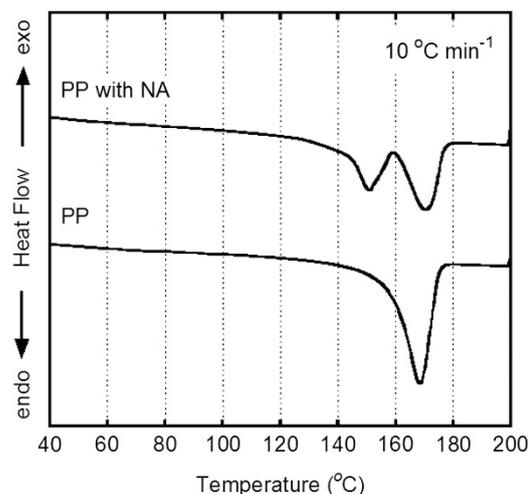
**Figure 1** Differential scanning calorimetry heating curves of injection-molded plates at a heating rate of 10 °C min<sup>-1</sup>.
