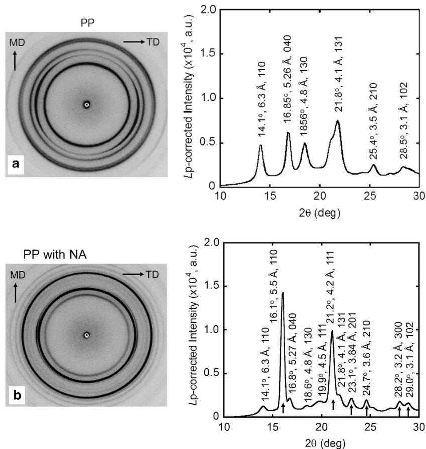
**Figure 3** Wide-angle X-ray diffraction (WAXD) patterns with the Lp-corrected curve of an entire plate of (a) pure polypropylene (PP) and (b) PP containing the nucleating agent. The  $2\theta$  angle,  $d$  spacing, and  $hkl$  indices are assigned in the figure, and the peaks attributed to  $\beta$ -form crystals are indicated by arrows in (b).
