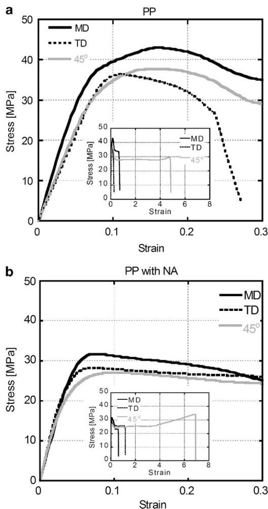
**Figure 7** Engineering stress-strain curves at various stretching directions of the injection-molded plates at room temperature: (a) pure polypropylene (PP) and (b) PP containing the nucleating agent. The strain rate is  $0.083 \text{ s}^{-1}$ .
