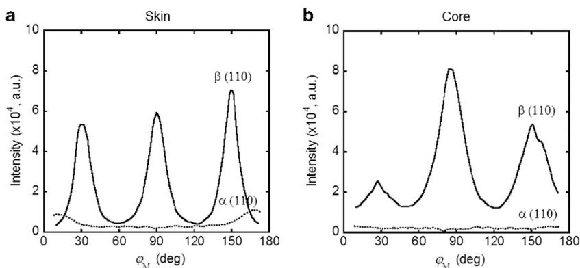
**Figure 5** Azimuthal intensity distributions of the (110) reflection of the  $\alpha$ -form crystal (dotted line) and the (110) reflection of the  $\beta$ -form crystal (solid line) vs  $\varphi_M$  of the plate containing the nucleating agent: (a) skin and (b) core layers.
