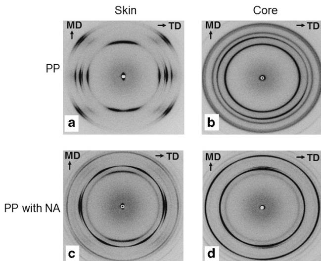
**Figure 4** Wide-angle X-ray diffraction (WAXD) patterns of injection-molded plates: (a) the skin layer for pure polypropylene (PP), (b) the core layer for pure PP, (c) the skin layer for PP containing the nucleating agent and (d) the core layer for PP containing the nucleating agent.
