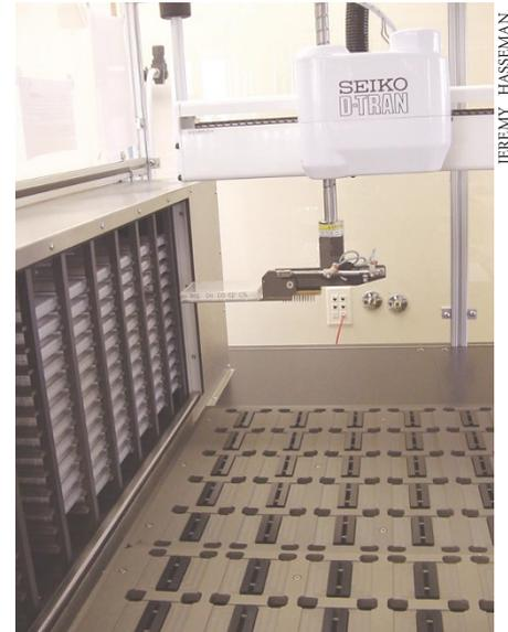
Custom-built robot arrayer in action at TIGR can spot 100 slides at a time.
