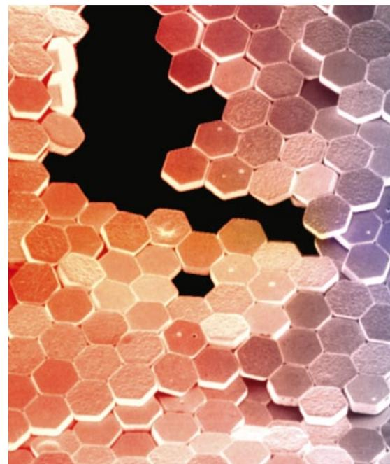
**Stuck up:** tiny gold tiles can be made to self-assemble in water into a range of structures by coating either the edges (above), faces (below) or both (left) with a water-repellent compound.
