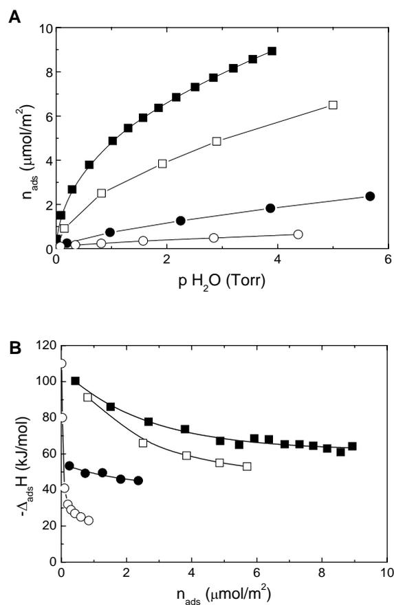
**Figure 6.** Adsorption of water vapor on the pyrogenic silica Aerosil 50 (round symbols) and the precipitated silica FK320 (square symbols): (A) amount of water adsorbed as a function of the equilibrium pressure; (B) enthalpy of adsorption as a function of water uptake. Samples were outgassed 2 h at either room temperature (full symbols) or 800°C (empty symbols) before water vapor adsorption at  $T = 30^\circ\text{C}$ .
