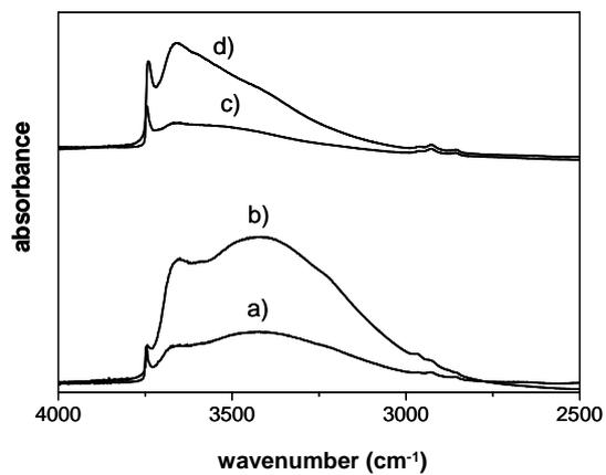
**Figure 7.** Effect of a hydrothermal treatment on silanol population of the pyrogenic silica Aerosil 50. FT-IR spectra in the hydroxyl stretching spectral region (4000-2500 cm<sup>-1</sup>) of Aerosil 50 before (spectra a and c) and after (spectra b and d) the hydrothermal treatment: (a) and (b) spectra recorded in air, (c) and (d) spectra recorded after outgassing 2 h at room temperature.
