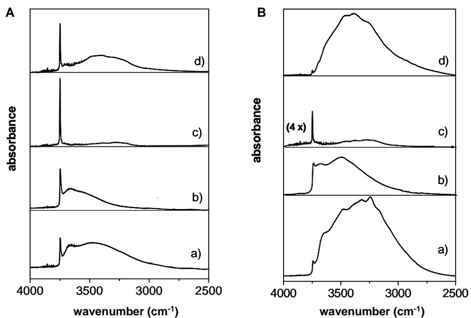
**Figure 5.** IR spectra of the pyrogenic silica Aerosil 50 (A) and the precipitated one FK320 (B) in the hydroxyl stretching spectral region ( $4000\text{-}2500\text{ cm}^{-1}$ ). Spectra of both samples were recorded in air (a); after outgassing 2 h at either room temperature (b), or  $800^{\circ}\text{C}$  (c); after outgassing at  $800^{\circ}\text{C}$  and in presence of water vapor pressure (ca. 20 Torr) at room temperature (d).
