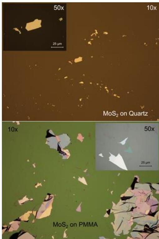
**Figure S2.** Examples of mechanically exfoliated MoS<sub>2</sub> flakes on quartz (top) and PMMA (bottom) substrates. The yield of exfoliation is very similar to that of graphene. WS<sub>2</sub> demonstrates very similar behavior.
