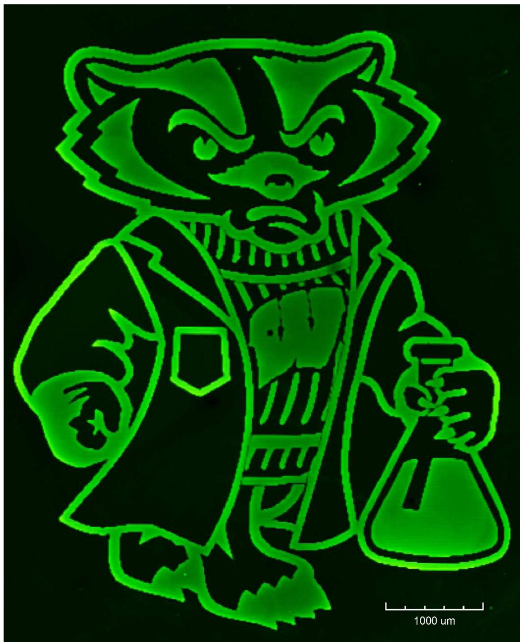
**Figure 8.** Fluorescence image of an amorphous carbon substrate after biotin immobilization via thioesterification followed by staining with fluorescently-tagged avidin.
