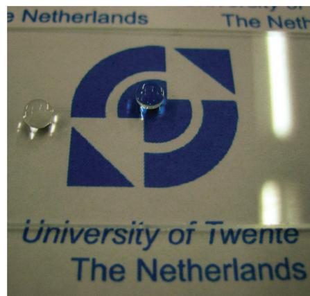
**Figure 6.** A photograph of water droplets on a superhydrophobic glass surface, prepared by the dip-coating method and functionalization with PFTS.
