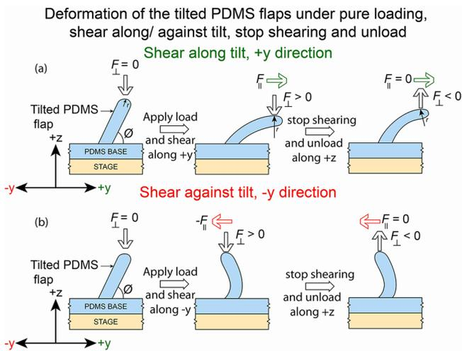
**Figure 3.** Schematics of a single flap deformation showing the separation of the flap with the upper silica surface after the flaps are sheared (a) along the direction of the tilt (+y direction) (b) against the direction of the tilt (−y direction). The adhesion forces,  $-F_{\perp}$  measured after sliding the top surface in the +y direction are significantly higher than the values measured after sliding in the −y direction.
