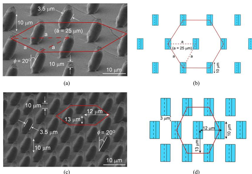
**Figure 1.** SEM images of the (a) low areal density ( $1850 \text{ flaps/mm}^2$ ), 1X tilted PDMS flaps and (c) high areal density ( $6410 \text{ flaps/mm}^2$ ), 3.5X tilted PDMS flaps. The flaps are tilted at an angle of  $20^\circ$  from the vertical. Schematic top-view orthographic diagrams showing the positions of the flaps relative to each other for both the (b) 1X flaps and (d) 3.5X flaps.
