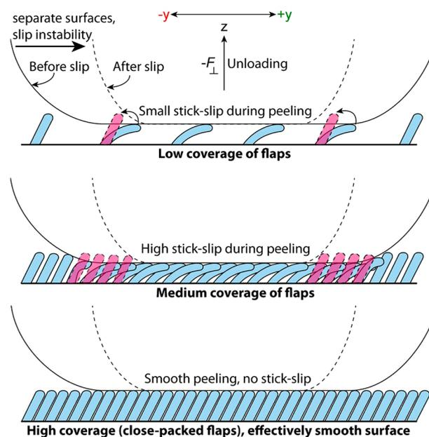
**Figure 7.** The magnitude of stick-slip instabilities observed in the load and friction forces (See Figures 6a and) during the peeling of the spherical glass disc from the patterned surface increases with increase in the flap density and would disappear eventually resulting in smooth peeling. This observation can be attributed to the number of flaps undergoing detachment during slip instability in the system. The flaps undergoing slip during instability are shown in red.
