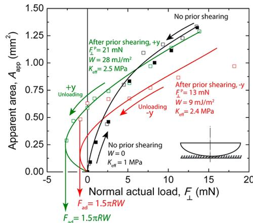
**Figure 4.** The apparent area,  $A_{\text{app}}$  vs the normal actual load,  $F_{\perp}$  for the 1X tilted PDMS microflaps as they are separated (unloaded) from the spherical silica surface of radius of curvature,  $R = 2$  cm. The open squares represent the experimentally observed  $A_{\text{app}}$  when unloading the flaps from the silica surface. The curves show the JKR fits to the experimental data.
