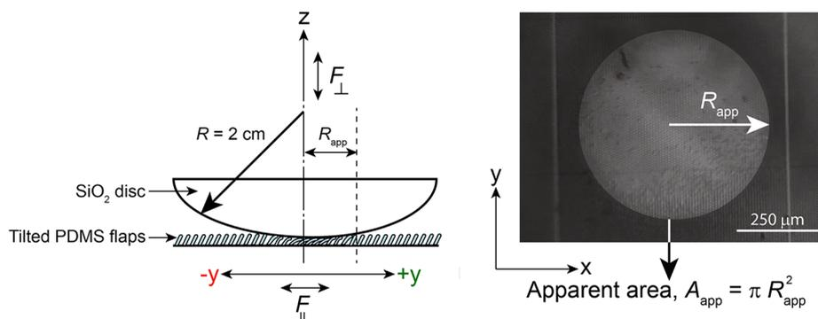
**Figure 2.** The apparent area,  $A_{app}$ , of contact when the arrays of PDMS microflaps are compressed against a spherical silica disc of radius of curvature,  $R = 2 \text{ cm}$ . The bright circular area\* shows the region of flaps that is in the deformed state. \*Contrast has been enhanced for clarity.
