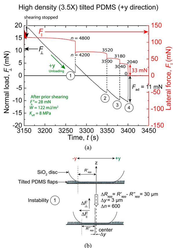
**Figure 6.** (a) Real time normal load and lateral force (friction) measurement of the high density (3.5X) tilted PDMS flaps against a spherical glass surface (RMS roughness = 1 nm) with prior shearing of the surfaces along the  $+y$  direction. Here,  $n$  gives the number of the tilted microflaps in contact with the glass surface just before and after the instability jumps. (b) Schematics of the contact just before and after the instability jump at 1.
