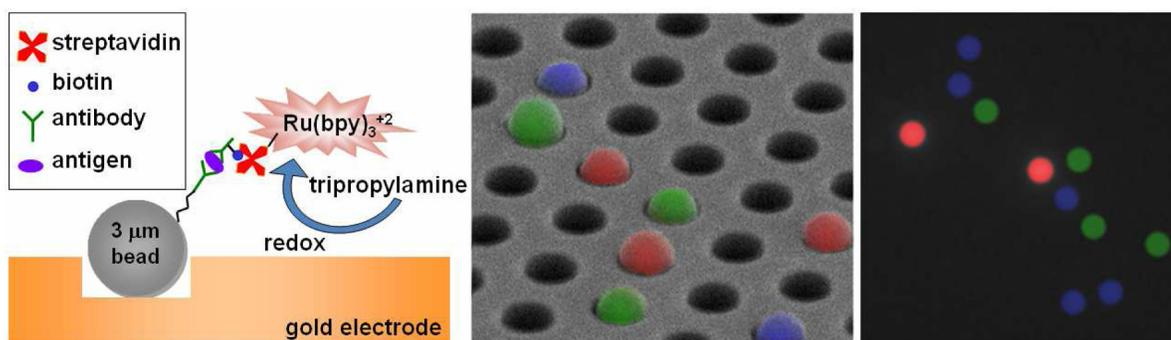
A new class of bead-based microarray that uses electrogenerated chemiluminescence (ECL) as a readout mechanism to detect multiple antigens simultaneously is presented. This platform demonstrates the possibility of performing highly multiplexed assays using ECL because all the individual sensing beads in the array are simultaneously imaged and individually resolved by ECL. Duplex and triplex assay results are demonstrated as well as a cross reactivity study.
