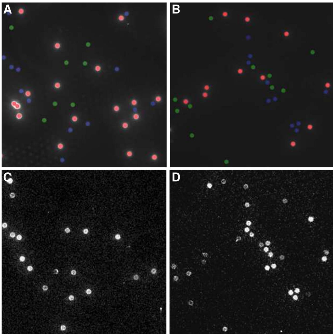
**Figure 3.** (A, B) Fluorescence images of two arrays containing anti-VEGF, IL-8, and TIMP-1 modified beads (false-color overlay with color scheme same as for Figure 2). (C) ECL image of the array in (A) following exposure to a sample solution containing both [IL-8] = 50 ng/mL and [TIMP-1] = 1.5  $\mu$ g/mL. (D) ECL image of the array in (B) following exposure to a sample solution containing [IL-8] = 50 ng/mL, [TIMP-1] = 1.5  $\mu$ g/mL, and [VEGF] = 1.5  $\mu$ g/mL
