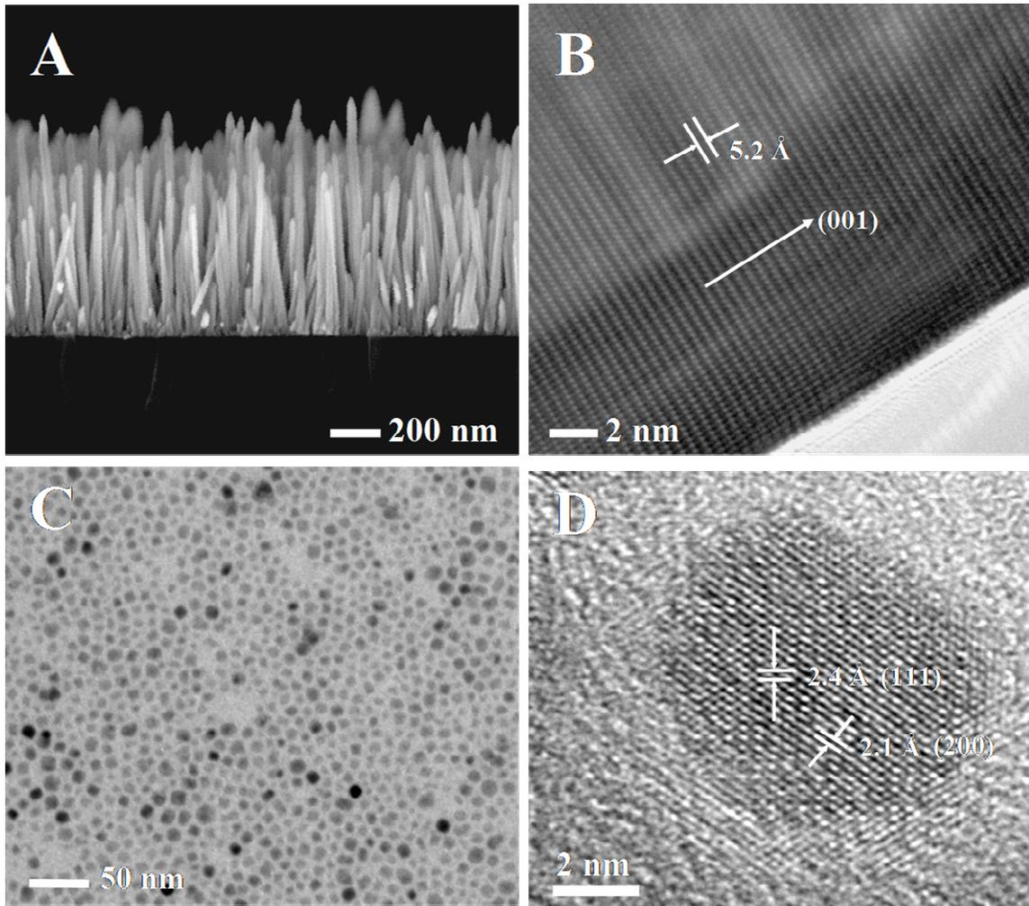
**Figure 1.** A) Cross-sectional SEM image of ZnO nanowire array used in solar cells, prior to Cu<sub>2</sub>O addition. B) High-resolution TEM image of an individual ZnO nanowire. C) Low r
