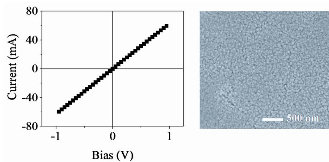
**Figure 6.** J-V Curve of a ZnO/Cu<sub>2</sub>O solar cell with no interceding TiO<sub>2</sub> layer, and corresponding top-down SEM image.
