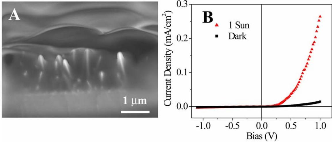
**Figure 2.** A) Cross-section SEM of a completed ZnO/Cu<sub>2</sub>O solar cell, with no Cu<sub>2</sub>O annealing performed. B) The corresponding J-V curve in darkness and under 1 Sun illumination.
