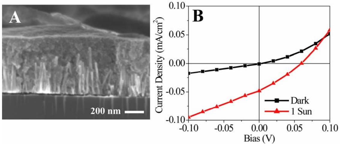
**Figure 4.** A) Cross-section SEM of a completed ZnO/Cu<sub>2</sub>O solar cell, with the cell annealed at 200°C after each application of Cu<sub>2</sub>O NPs. B) The corresponding J-V curve in darkness and under AM 1.5 and 1 Sun illumination.
