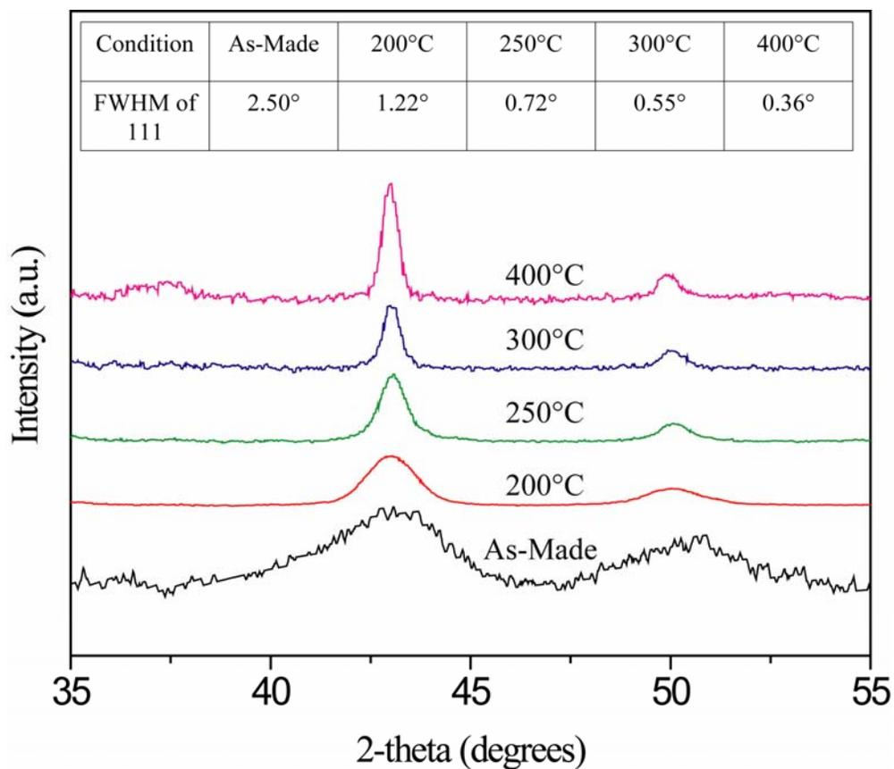
**Figure 5.** XRD patterns of  $\text{Cu}_2\text{O}$  NPs films on glass, annealed at the noted temperatures under 500 mTorr oxygen (Total pressure = 5 Torr). The patterns are vertically offset for clarity, and the accompanying table lists the measured FWHM values for the 111 peak at the different annealing temperatures.
