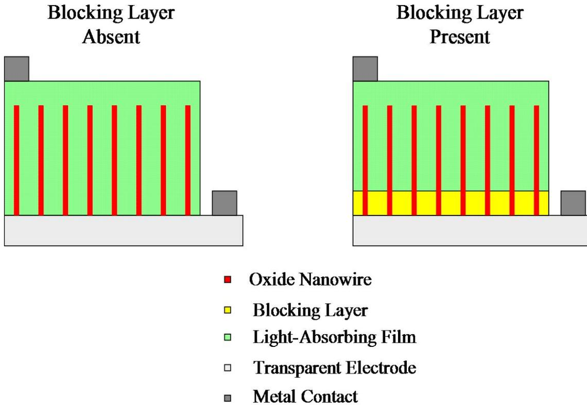
**Figure 8.** Illustration of a nanowire-based solar cell, with and without a blocking layer between the light-absorbing material and the transparent electrode. A shunt pathway exists for the case without a blocking layer, where it is absent in the case with the blocking layer.
