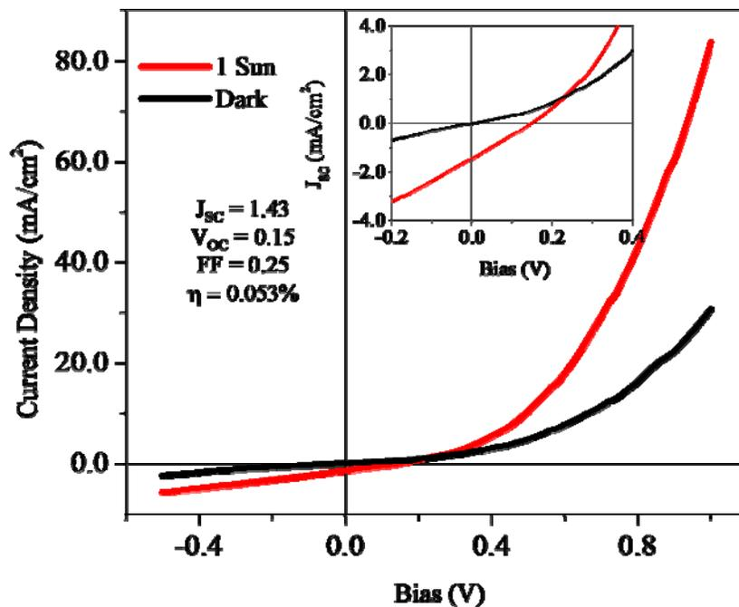
**Figure 7.** J-V curves of a ZnO/TiO<sub>2</sub>/Cu<sub>2</sub>O solar cell in darkness and under 1 Sun illumination. The Cu<sub>2</sub>O film was annealed at 300°C under 500 mTorr oxygen. The ZnO NWs are 500 nm in length, the TiO<sub>2</sub> coating layer is 10 nm thick, and the Cu<sub>2</sub>O film thickness is 800 nm.
