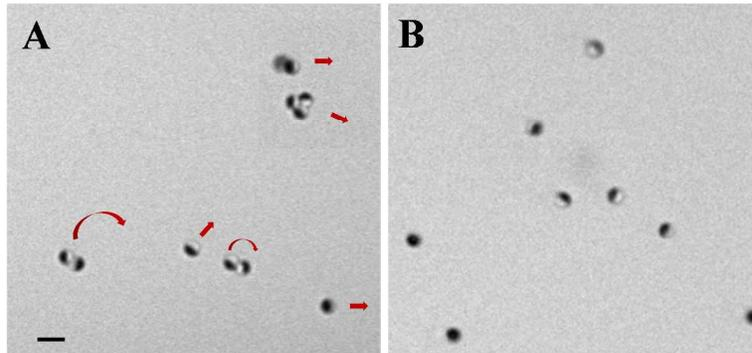
**SI Figure 1.** Control experiments (taken from SI Video 3): Janus micromotors with (A) and without (B) hydrophobic coating. The latter offers simultaneous movement of single, doublet, and triplet motor assemblies. Scale bar, 2  $\mu\text{m}$ . Conditions, as in Figure 1.
