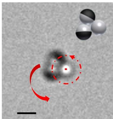
**SI Figure 5.** Motor/non-motor interaction: rotational motion with the non-motor anchored to the glass surface (taken from SI Video 7). Scale bar, 2  $\mu\text{m}$ . Conditions, as in Figure 1.
