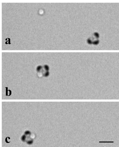
**SI Figure 3.** ‘On-the-fly’ capture of a non-motor particle by a triplet micromotor assembly. Time-lapse images of a, b, and c have been taken from SI Video 6 in 1 second intervals. Scale bar, 3  $\mu\text{m}$ . Conditions, 5% hydrogen peroxide.
