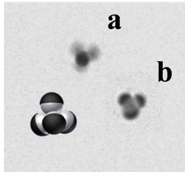
**SI Figure 2.** Self-propelled tetrahedral structure based on the assembly of four Janus micromotors: (a) and (b) show optical microscope images of the same tetrahedral structure at different times (taken from SI Video 4). Conditions, as Figure 1.
