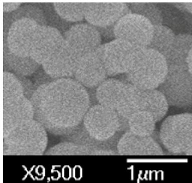
**Supporting Figure 2.** SEM image of calcined mesostructured amine-modified silica nanoparticles.
