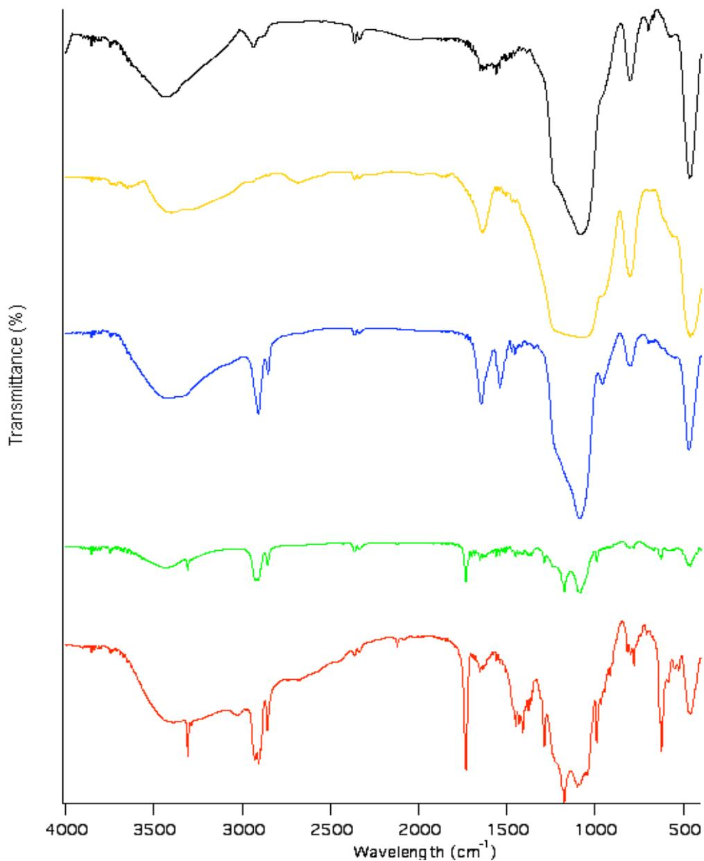
**Supporting Figure 3.** FTIR spectra of amine particles (**black**), azide particles (**orange**), amide-capped particles (**blue**), ester-capped particles (**green**) and released ester-capped particles (**red**)
