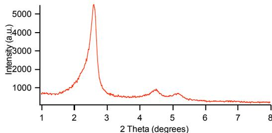
**Supporting Figure 1.** XRD pattern of calcined mesostructured silica nanoparticles. The 100 peak at  $2\theta = 2.6^\circ$  corresponds to a 2D-hexagonal mesostructure with lattice spacing of 3.4 nm.
