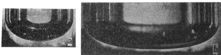
Fig. 8.—Benzene in tubes ( a ) of 6 mm. and ( b ) of 12 mm. diameter magnified 5 diameters. Very little distortion of the image appears in these photographs, so that they give nearly the true profiles of the meniscuses; ( a ) is essentially elliptical, falling on Desains's curve; ( b ) is of the nondescript type treated only by our experimental curve (See Fig. 5).
