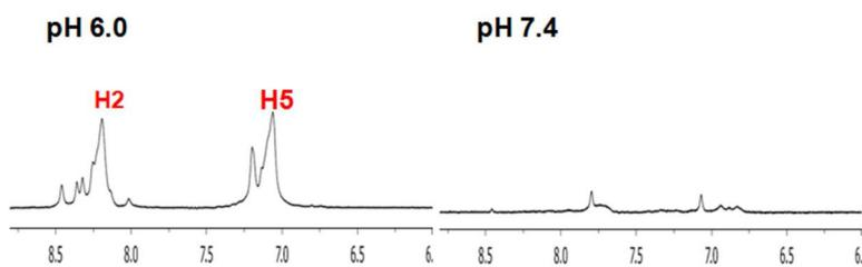
**Figure 5.**  $^1\text{H-NMR}$  spectra of H2 and H5 peaks in mixed micelles of  $\text{PEG}_{2\text{kDa}}\text{-PHis}_{3.3\text{kDa}}$  (90 wt.%) having  $\text{PEG}_{2\text{kDa}}\text{-PLLA}_{3\text{kDa}}$  (10 wt.%) exposed at two different pHs (pH 7.4 and pH 6.0) of rat whole blood.
