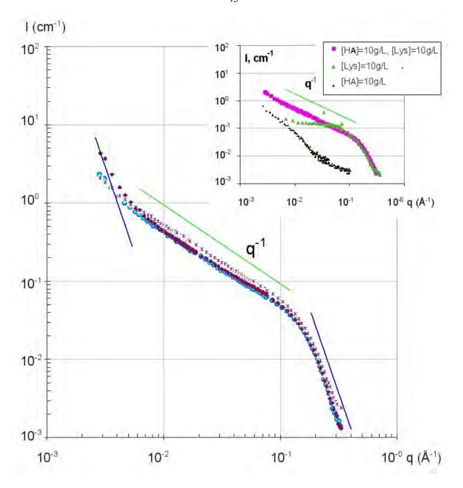
**Figure 5.** SANS I(q) (not normalized by concentration) as a function of q presenting a large  $q^{-1}$  domain for 3 complexes HA2 (large mass, 10g/L), and lysozyme:  $\bullet$ : 8, \*: 10,  $\bullet$ : 15 g/L, pH = 4.7 shown already in **Figure 2**. Inset: comparison between HA/lysozyme 10g/L/10g/L, pure lysozyme and pure HA2 at the same concentrations.
