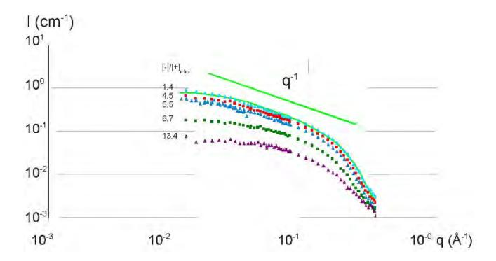
Figure 8. SANS scattering as a function of q for sample of HA1 (small mass, 10g/L) and lysozyme:  $\triangle:3g/L$ ,  $\blacksquare:8g/L$ ,  $\triangle:27g/L$ ,  $\blacksquare:40g/L$ ,  $\triangle:40g/L$  (shaken) in buffer solution at pH = 7.4. In solid line (green), a fit, for  $C_{lyso} = 40$  g/L, of a rod scattering, length 15 nm, average radius 1.1 nm, volume fraction 0.252, and average contrast  $\Delta \rho^2 = 4.18 \ 10^{10}$  cm<sup>-4</sup>.
