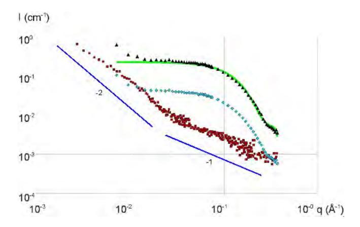
**Figure 1.** SANS I(q) as a function of q for pure HA2 (large mass) solution (■ 10g/L,) and pure lysozyme solution (♦ 3.32 g/L and ▲ 20 g/L) in buffer at pH 7.4. In solid line (green), a fit of the lysozyme signal with the form factor of a polydisperse sphere of radius 1.55 nm.
