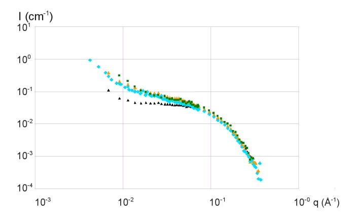
**Figure 4.** SANS scattering I(q) in buffer at pH = 7.4 for a lysozyme solution (  $\blacktriangle$ : 3.32g/L) and mixtures of HA2 (large mass, 10g/L) and lysozyme ( $\blacksquare$ :3.32g/L,  $\blacktriangleleft$ :6.64g/L,  $\spadesuit$ :8g/L (liquid phase), corresponding to the three lowest curves of **Figure 2** and divided - for comparison at same lysozyme concentration- respectively by 1, 2, as expected, and 2 (instead of 2.4 = 8/3.32).
