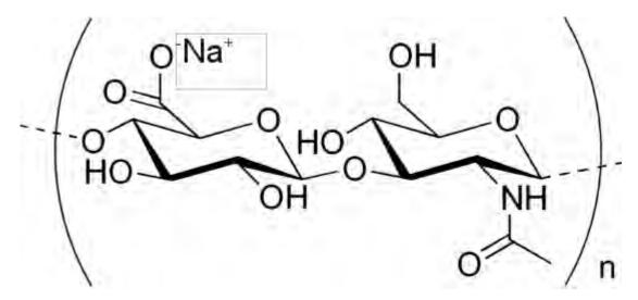
**Scheme 1.** Chemical structure of hyaluronan. The length of the segment is 1 nm.
