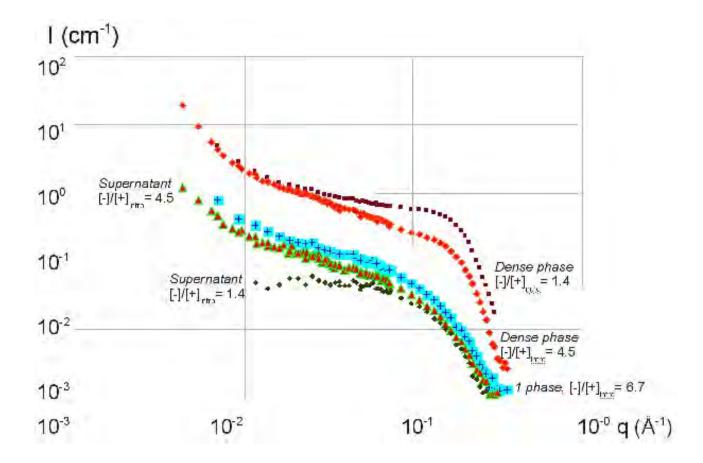
**Figure 6.** Comparison of supernatant and dense phase: SANS scattering I(q) for mixtures of HA2 (large mass, 10g/L) and lysozyme:  $\stackrel{\bullet}{+}$ : 6.6g/L, monophasic  $\stackrel{\bullet}{\triangle}$ ; and  $\stackrel{\bullet}{\bullet}$  are respectively supernatant and dense phase of 10g/L,  $\stackrel{\bullet}{\bullet}$  and  $\stackrel{\bullet}{\bullet}$  are respectively supernatant and dense phase of 40g/L, at pH=7.4.
