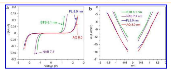
Figure 6. (a) JV curves of BTB, NAB, FL, and AQ with thicknesses close to 8 nm. (b)  $\ln |J| vs V^{1/2}$  plots for curves in panel a.
