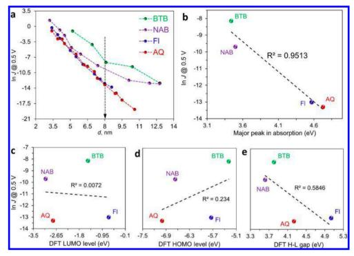
Figure 7. (a) Attenuation plots for BTB, NAB, FL, and AQ, all obtained at 0.5 V. (b) ln J for V = 0.5 V and d = 8 nm for the four molecules plotted vs the energy of the main UV-vis absorption peak of the molecular layer shown in Figure 4d.  $R^2$  is the correlation coefficient for the linear fit shown. (c) The same ln J plotted vs the DFT determined LUMO energy of the free molecules (d) ln J vs free molecule HOMO energy from DFT. (e) ln J vs the DFT determined HOMO-LUMO gap.
