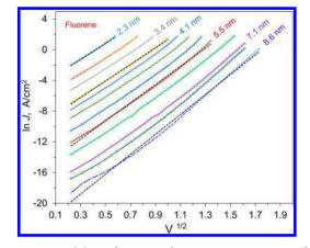
Figure 3. Natural log of current density vs square root of bias voltage for the same series of FL junctions shown in Figure 2, for positive bias. Order of thickness is the same as in Figure 2a.
