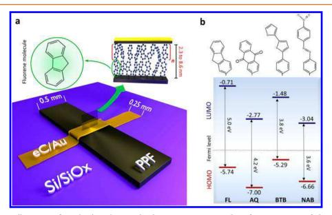
Figure 1. (a) Schematic illustration of PPF/FL/ $eC_{10}/Au_{20}$  molecular junction; *n* is a number of repeating units of oligomer that determines final thickness of molecular layer. (b) Structures and frontier orbital energy diagram for FL, AQ, NAB, and BTB, relative to a vacuum reference. Orbital energies were calculated by DFT B3LYP 6-31G(d), in Gaussian 09. Fermi level of PPF and eC is -4.8 V vs vacuum.
