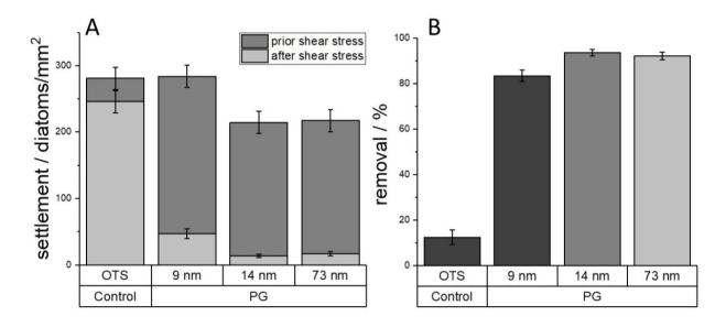
Figure 5. A: The density of settled diatoms on the controls and PG surfaces after 2 h. The bright parts of the bars indicate the density of diatoms remaining on PG surfaces after exposure to a shear stress of 19 Pa. Each data point is the mean from 90 counts on three replicate slides. Error bars show the 95 % confidence limits. B: Percentage removal of diatoms from PG surfaces by the
