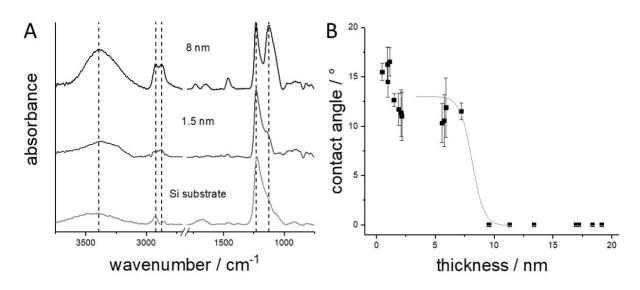
Figure 3. A: ATR-FTIR spectra of two different thicknesses of PG (8 nm and 1.5 nm) and a blank silicon wafer as a control. Three vibrational modes indicate formation of the PG, which are the ether stretch vibrations at 1127 cm<sup>-1</sup>, C-H stretch vibrations at 2923 cm<sup>-1</sup> and 2875 cm<sup>-1</sup>, and
