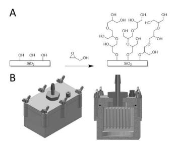
Figure 1. A: Summary of the ring-opening polymerization (ROP) of glycidol on a hydroxylated silica surface. The OH groups of the silicon oxide act as a nucleophile and can promote the grafting process of the dendritic polyglycerol (PG). B: Teflon reaction vessel developed for the ROP synthesis of PGs on glass slides under a
