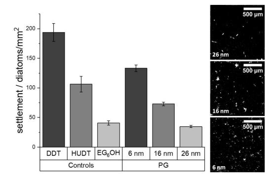
Figure 6. Comparison of the performance of the three SAM controls (DDT, HUDT, EG<sub>6</sub>OH) and three thicknesses of PG in the dynamic field test in Florida. Each data point is the average of 240 counts of diatoms on four replicate slides. Error bars represent the standard error of the mean.
