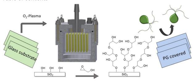
Dendritic polyglycerol coatings prepared via surface initiated ring-opening polymerization were discovered as marine fouling-release coatings.
