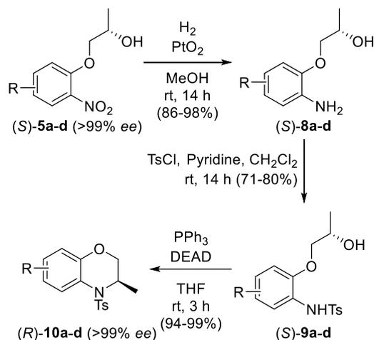
**Scheme 3.** Chemical synthesis of protected enantiopure benzoxazines **10a-d**.
