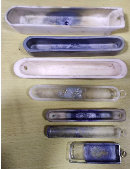
Figure S7: Optical image of crucibles (boats) used in the synthesis of  $\text{MoS}_2$  for controlling the  $s$ ,  $d$  and  $h$  to play with concentration boundary layer.
