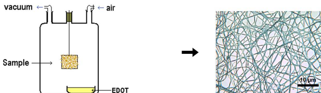
Figure 1. Scheme of the two-step nanofiber production. On the right-side are optical micrographs of the resulting nanofibers (reflection mode for step 1 and transmission mode for step 2).
