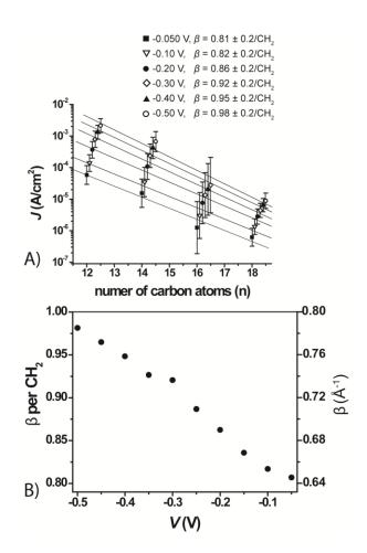
**Table 1:** Fitting Results<sup>a</sup> to Plots of the Value of *J* as a Function of the Number of Carbon Atoms in the SAM.
