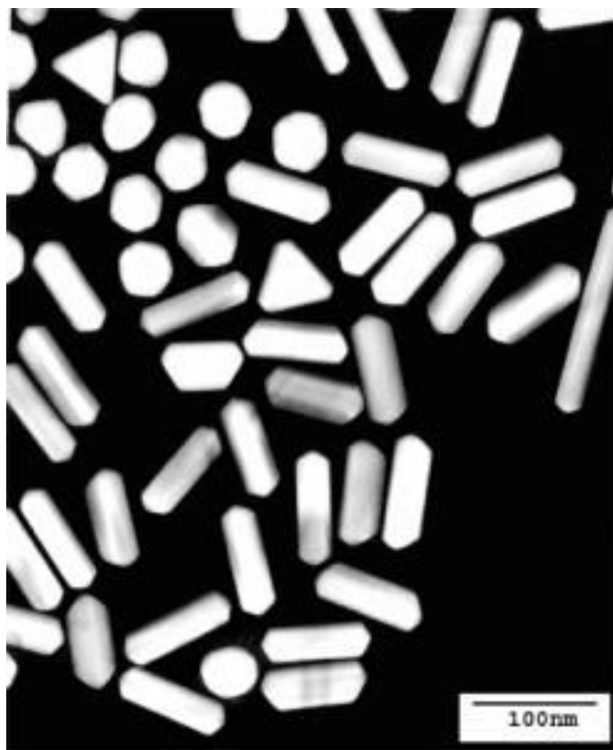
Figure 6. TEM image (Philips CM-10, 80 kV) of anisotropic Au nanoparticles prepared in the absence of \text{AgNO}_3 , followed by quenching with \text{Na}_2\text{S} ( t = 25 min). Nanorod suspensions were subjected to one C/R cycle prior to sample preparation.
