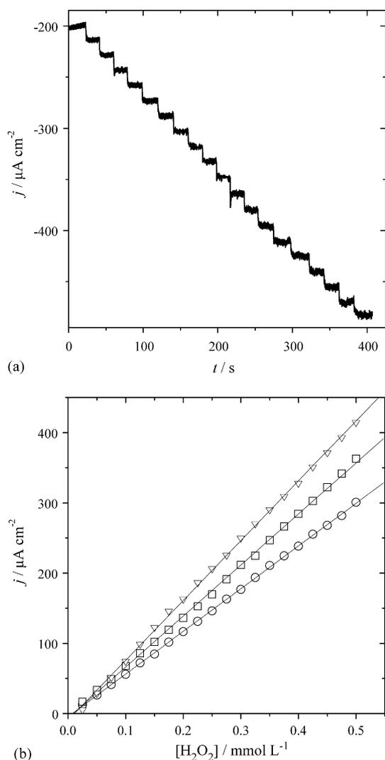
Fig. 2. (a) Typical amperometric response during the determination of  $\text{H}_2\text{O}_2$  with a PPy/CuHCNFe hybrid glassy carbon modified electrode at 0.0 V vs. SCE. (b) Analytical curves obtained for  $\text{H}_2\text{O}_2$  determination at 0.0 V vs. SCE in  $0.1 \text{ mol L}^{-1} \text{ KCl} + 0.1 \text{ mol L}^{-1} \text{ HCl}$  with a PPy/CuHCNFe hybrid glassy carbon modified electrode.
