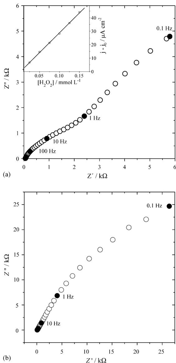
Fig. 4. Complex plane impedance spectra at  $0.0 \text{ V}$  vs. SCE of (a) a GC/CuHCNFe/PPy electrode after being partially overoxidised. The insert corresponds to the analytical curve obtained with the hybrid electrode after the partial overoxidation of the polypyrrole. (b) A GC/CuHCNFe/PPy electrode after being totally overoxidised till  $1.0 \text{ V}$ .
