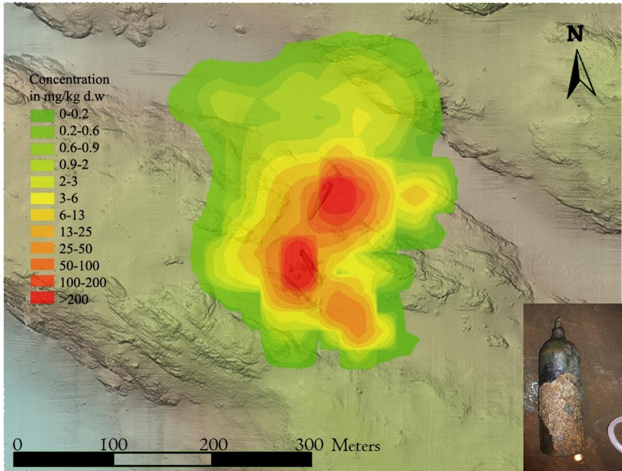
Figure 4. Mercury contamination on the U-864's seabed site and a photo of a corroded and leaky 2.5 L steel Hg canister recovered at the site. At the time of sinking, U-864 is estimated to have been carrying about 67 t of liquid Hg in about 860 metallic canisters like the one shown above.
